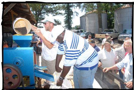
Canola seed is dumped into mechanical press. Oil and cake are the two byproducts.
