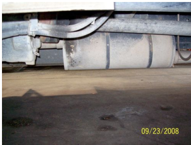
Figure 2: Muffler before DOC installation
