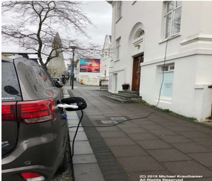
Figure 53. Example of problematic curbside charging in Washington, DC Credit: EV Advisors
