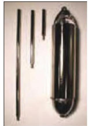
Bacon Bomb with extension rods to sample from tank bottoms. The (4 oz.) 1" diameter one is also referred to as the Pencil Bomb.
