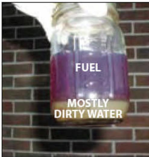
By the sample drawn above, this tank has a problem with excessive water accumulation. You can also detect this much water with water-indicating paste on a stick.
